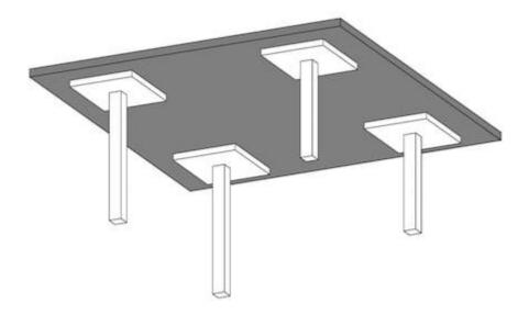
The flat plate slab does not have much structural capacity. There will be higher bending moments and shear forces around the column. When the uniformed slab thickness is not adequate, we increase the slab thickness. It increases the bending and shear resistance
