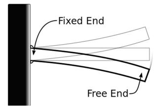
In the ideal condition, there will be no ration in at the support when the beam is supported on a fixed support.
